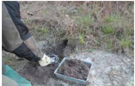
Figure 7. Poly-fill added under trap pan.
