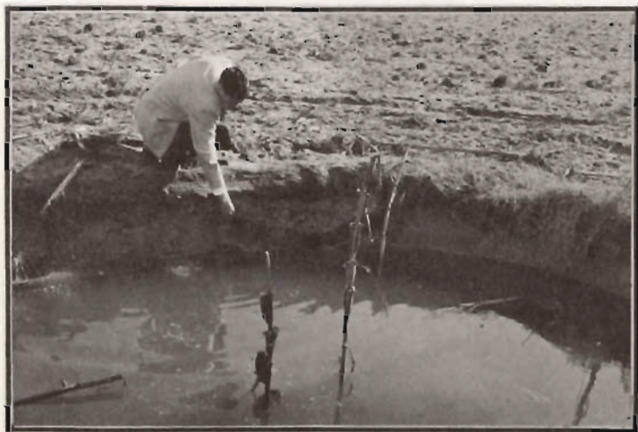
B. POINTING OUT BURIED TOPSOIL LAYER INDICATING SMALL SINKS IN THE PAST.
