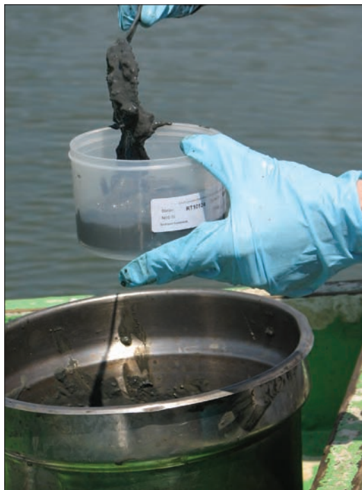
Placing a sediment composite sample in a container.
