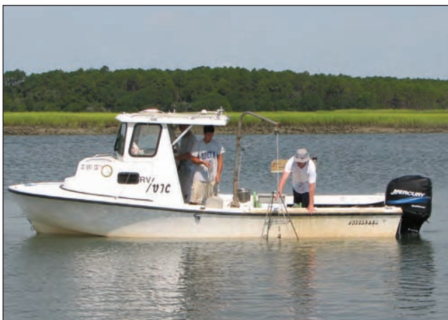
Deploying a grab sampler to collect a sediment sample for chemistry and benthic analysis.
