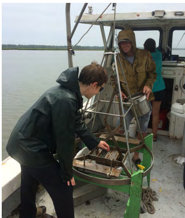
A Young grab is used to collect samples for sediment quality and benthic biological condition.
