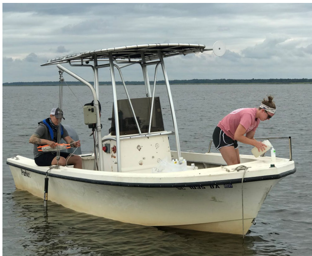
Near-surface water samples are collected to measure concentrations of nutrients, chlorophyll a , and fecal coliform bacteria.
