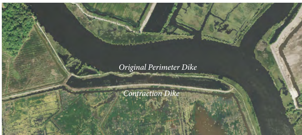
Example of a contraction dike replacing a failed or failing perimeter dike.
