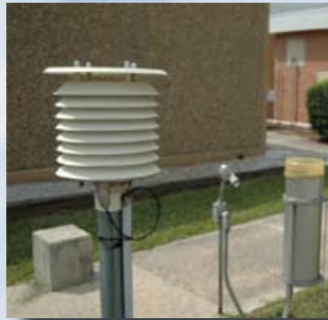
Modern cooperative weather observation station.
