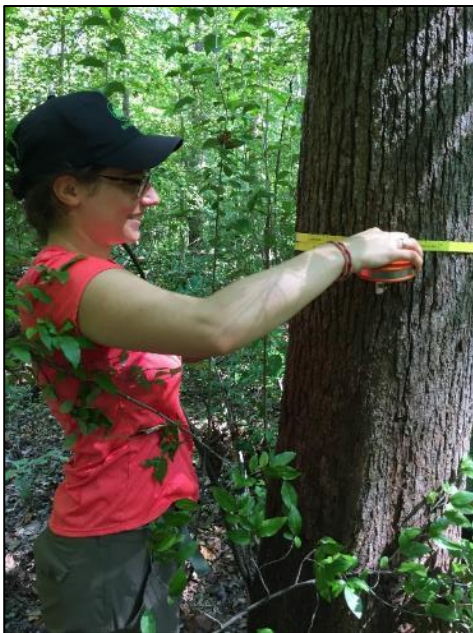
Figure 14. Measuring DBH (1.37 m or 4.5 feet above ground level).
